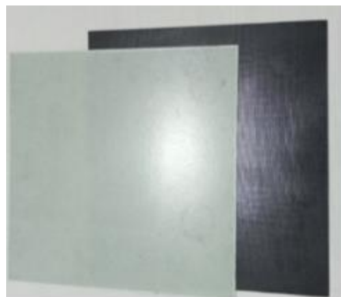
Fig. 1. Fibreglass and carbon fibre composite patches made under vacuum
