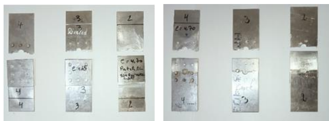
Fig. 24. Damage to the notched plates repaired by an aluminium patch using hybrid repair processes (bonding/riveting)
