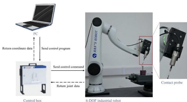
Fig. 8. Probing tool of robotic arms for quality control [147]
